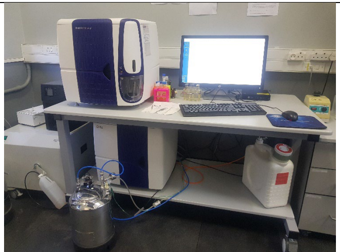
j. Becton Dickinson FACSMelody flow cytometer at the Central Analytical Facilities Fluorescence Microscopy Unit Main campus, Department of Physiology Stellenbosch University used for analysis of samples.
