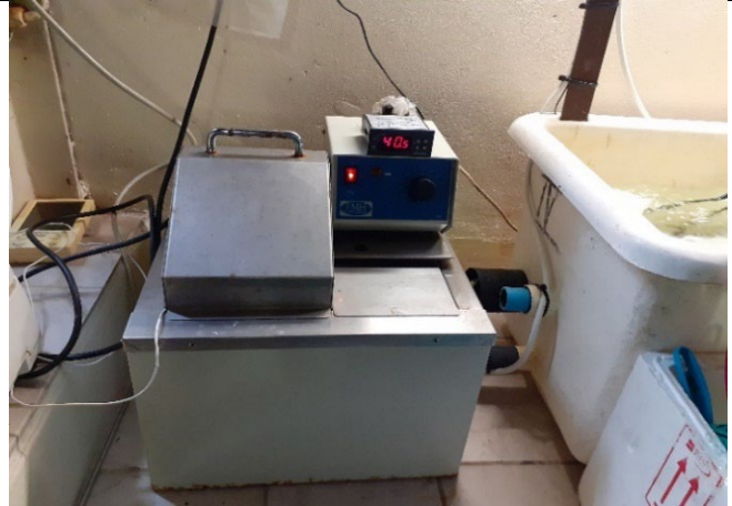
f. Heat-shock inducing warm water bath at 40.5°C in which treatment brushes are transferred the incubation tank.
