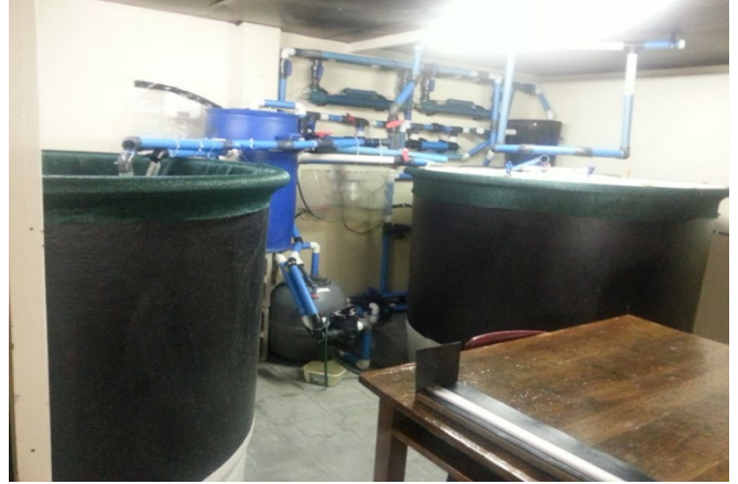
h. The RAS for keeping broodstock and larvae.
