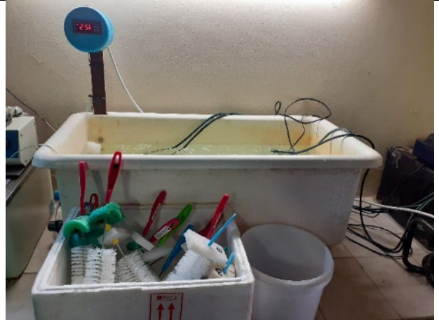
d. The warm-water bath set up at 25°C for incubation of embryos prior to the induction procedures.
