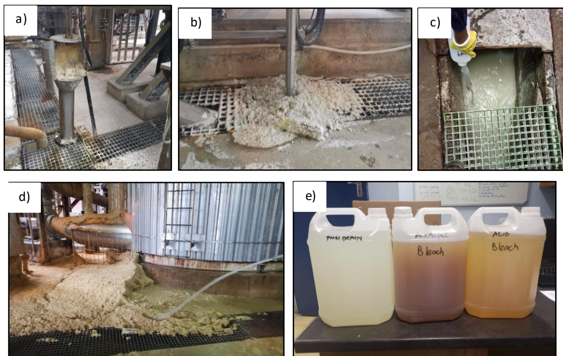
Figure 24: Sources of fibre waste from a Kraft pulp and paper mill a) sampling point spill, b) spill from drain valve or corroded pipe leak c) paper machine drain containing ‘white water’, d) tank overflow and e) collected samples from drains (left to right: PM41, Alkaline and Acid Effluent).
