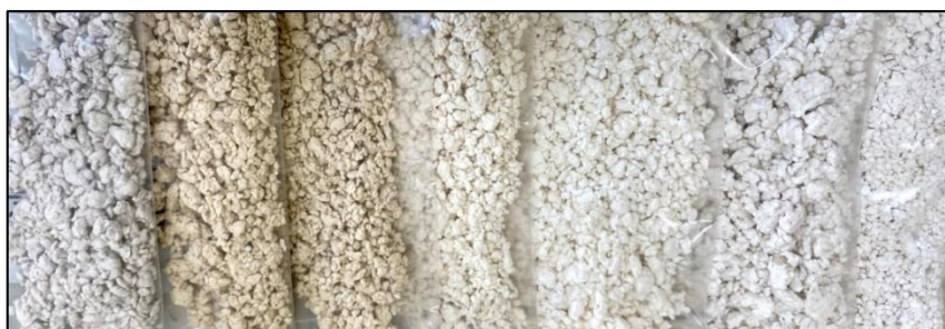
Figure 26: Freeze-dried fibre showing the difference (from left to right) in pulp color as bleaching progresses. From left to right: Broke Well, Bleach Spill, Dual D, OP, D1, D1/D2 and D2.
