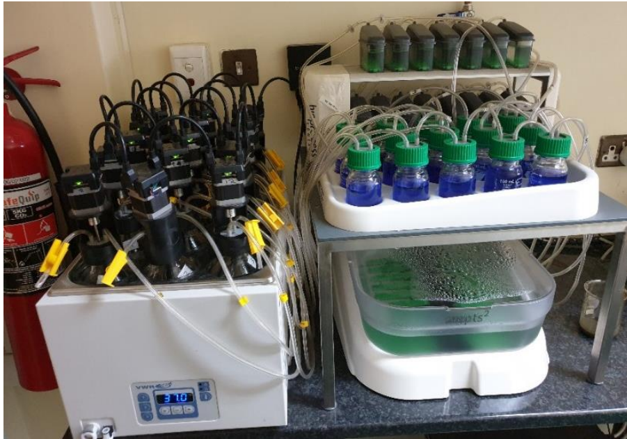
Figure 15: Photograph of the bench-scale AMPTS II setup, used for BMP assay tests.
