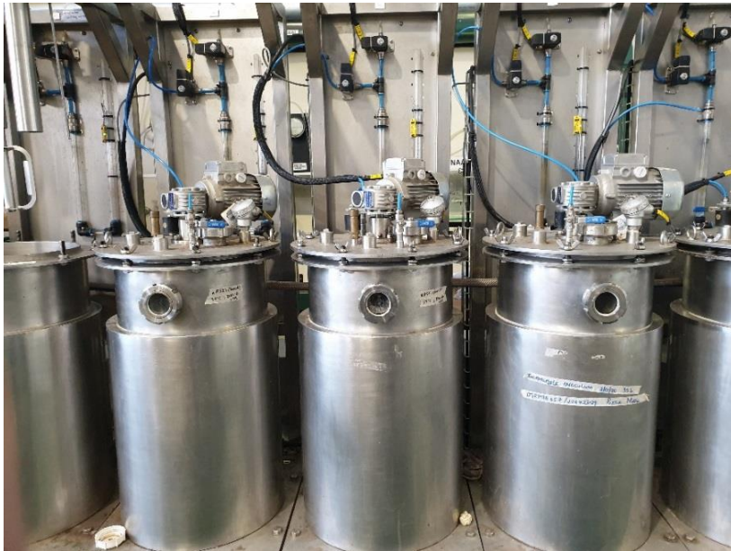
Figure 17: Photograph of the pilot-scale (50L) anaerobic digesters.
