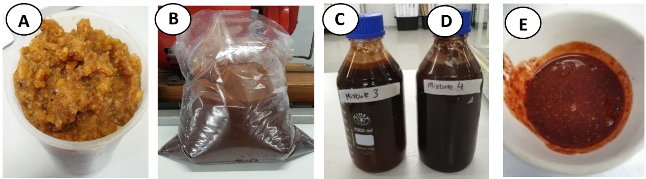
Figure 11: Photographs of feedstock mixtures obtained from Plant 1: (a) Mixture 1 (apples, food waste), (b) Mixture 2 (food waste, spices & beer), (c) Mixture 3 (food waste, spices, beer, cattle blood & manure), (d) Mixture 4 (chocolate processing waste, beer, sugar and cattle blood), (e) Mixture 5 (food waste, beer, fruit juice and cattle blood).
