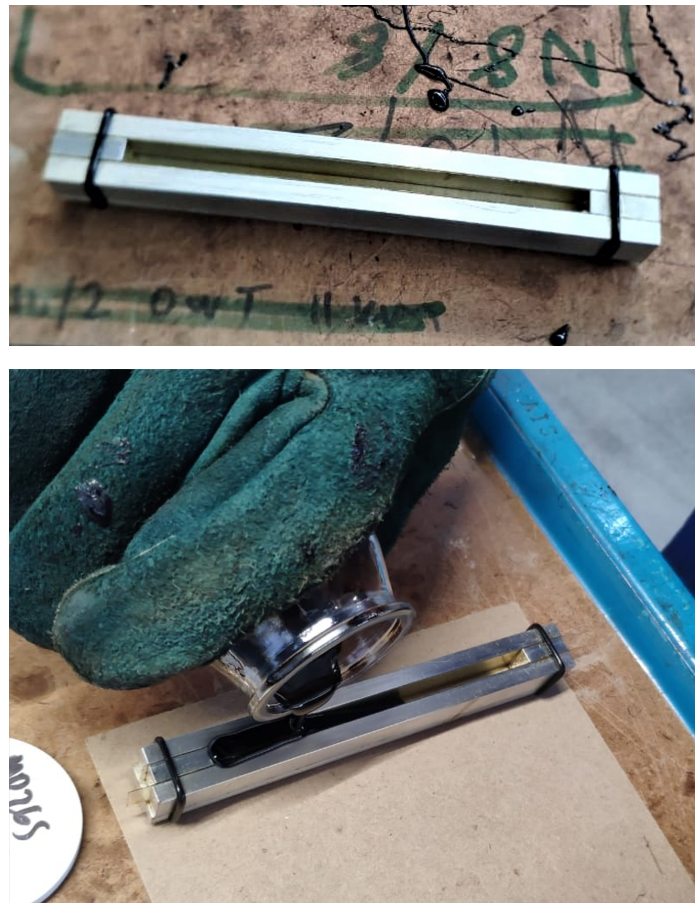
Figure 3.5: The empty constructed beam and the slow pouring of the binder into the beam
