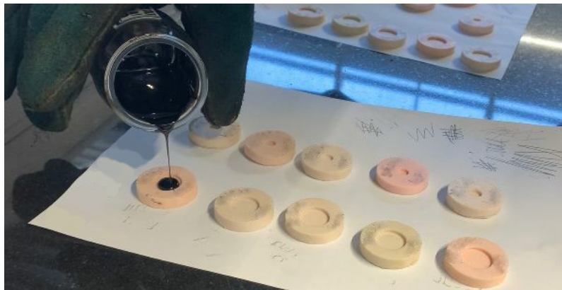
Figure 3.3: Pouring the binder into the moulds
