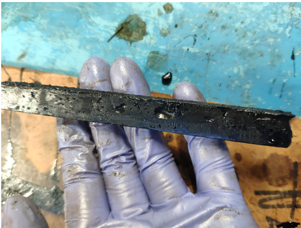
Figure 3.9: Beam with voids
