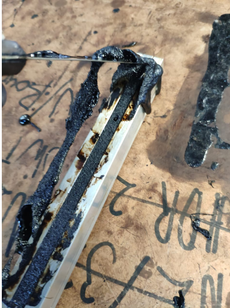
Figure 3.7: Trimming rubber beam
