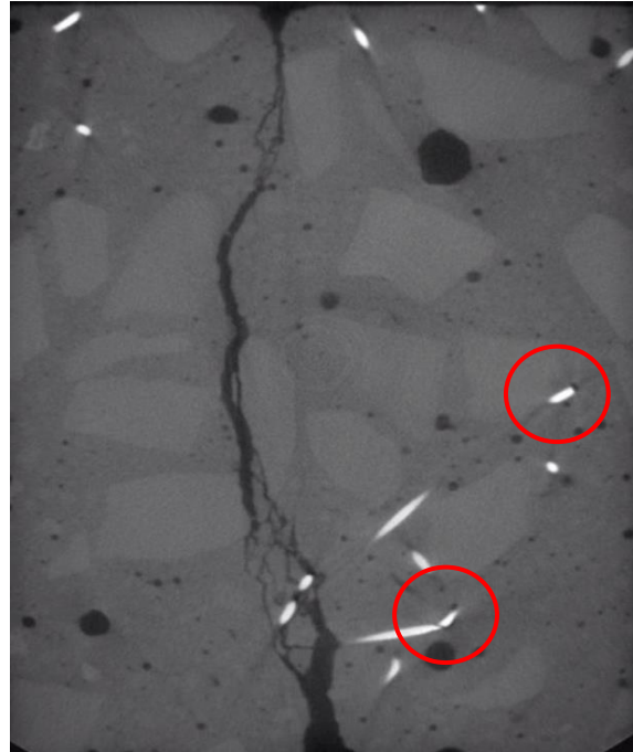
Figure 5.18: Post-fatigue test X-ray CT image of Specimen 3 tested to failure at 85% load level and 2.5 mm pre-crack showing fibre rupture and fibre pull-out
