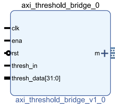
Figure B.5: AXI Threshold Bridge IP module
