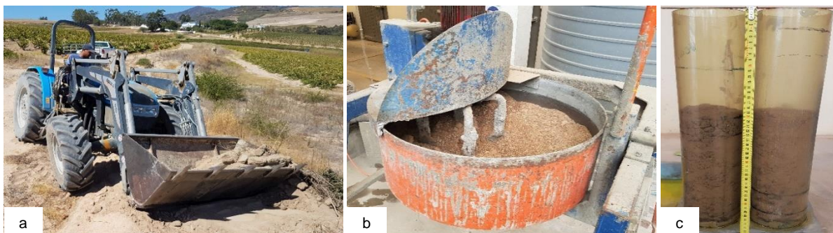
Figure 1.2a-c Soil excavated for experimental use, the 100 L pan mixer for uniform soil conditions, and perspex columns for infiltration.
