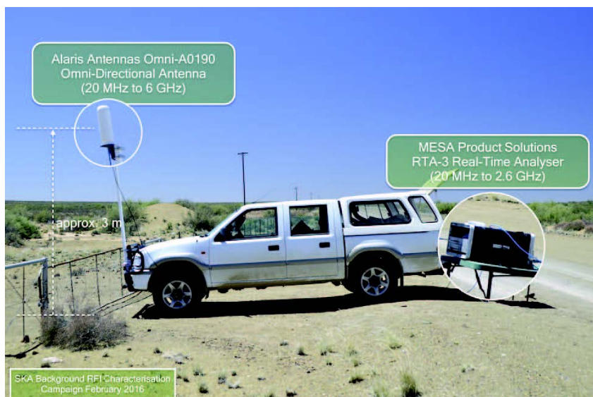
Figure 1.2: Setup for characterising environmental RFI at SKA1-MID [5]
