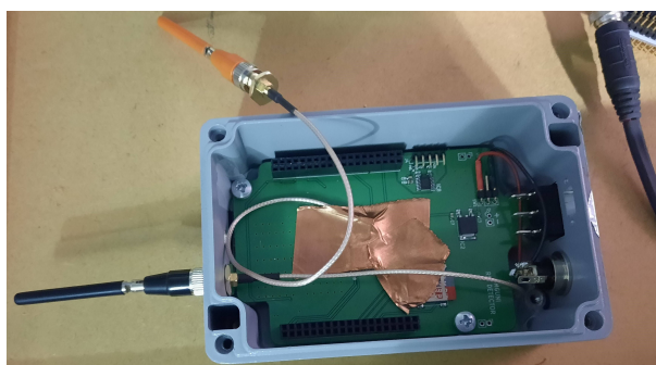
Figure 6.5: A picture of the RFIPD setup when enclosure is open with shielding over the GNSS receiver and the GNSS antenna removed from it's hole
