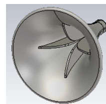
(b) CST model of a quad ridged flared horn [3]
