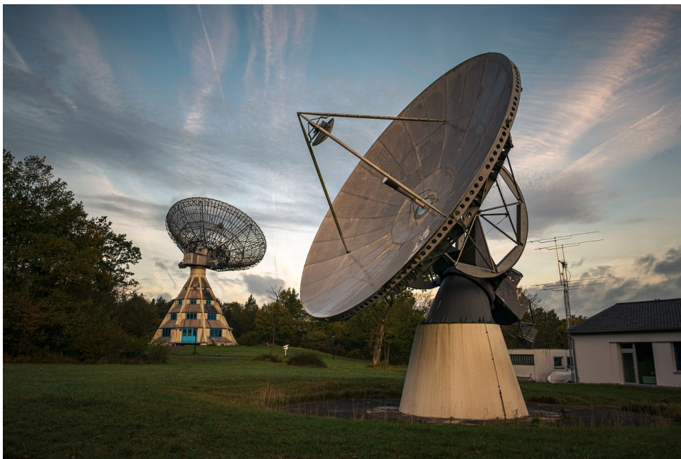
Figure 1.1: Photograph of a pair of Cassegrain dual reflector antennas used at the Stockert observatory in Eifel, Germany [1].
