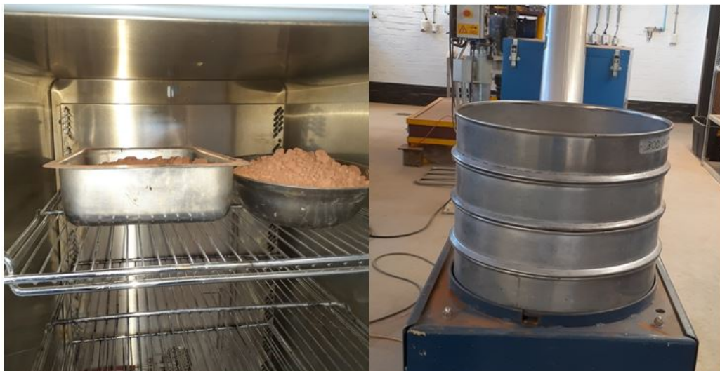
Figure 3.4: Oven drying aggregates and sieving
