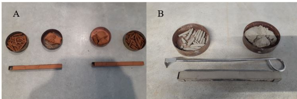
Figure 3.7: Linear shrinkage of Laterite and Crushed Stone materials
