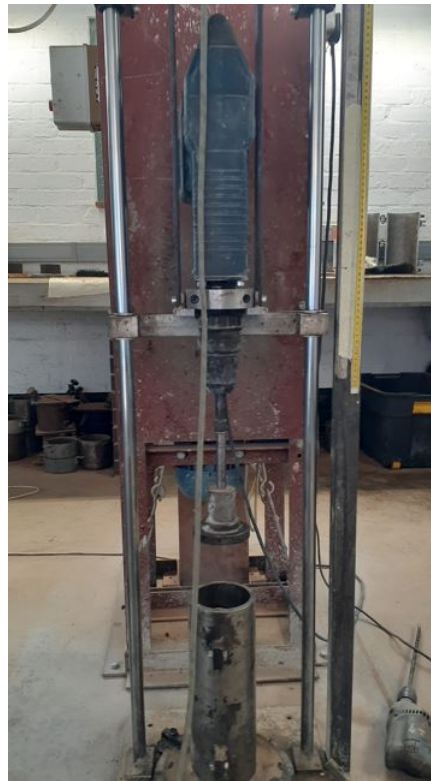
Figure 3.22: Vibratory hammer used to compact HPP samples
