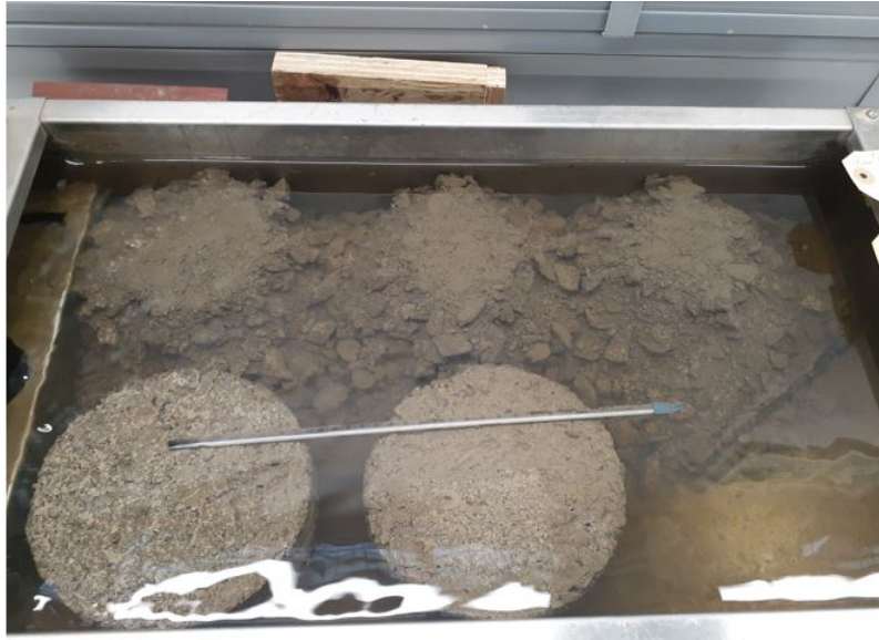
Figure 4.11: ITS_{WET} Kalumbila GCS base mix test specimens disintegrated in water
