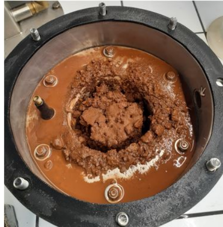
Figure 4.22: Laterite HPP results at 100 kPa
