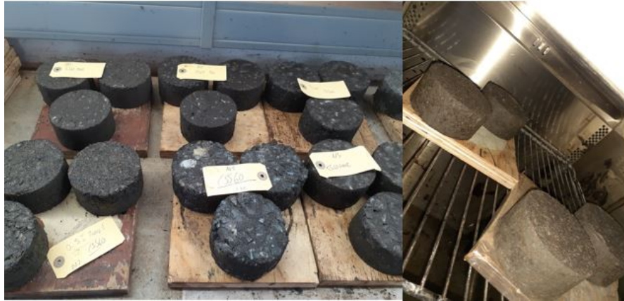
Figure 3.23: Compacted HPP samples and their curing.
