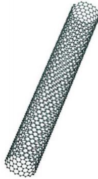
Figure 2.15: The structure of a carbon nanotube (CNT). (Mann, 2006)
