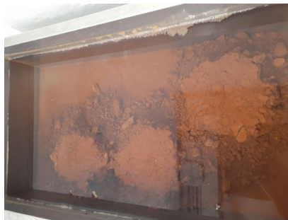
Figure 4.9: ITS_{WET} laterite base mix test specimens disintegrated in water
