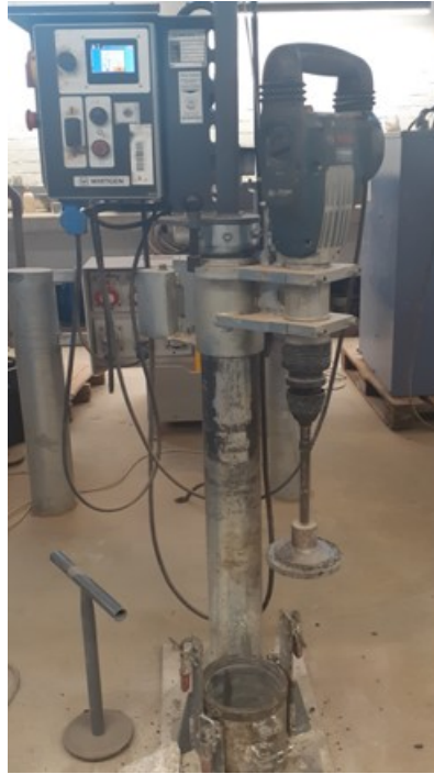
Figure 3.13: A vibratory hammer used for compaction
