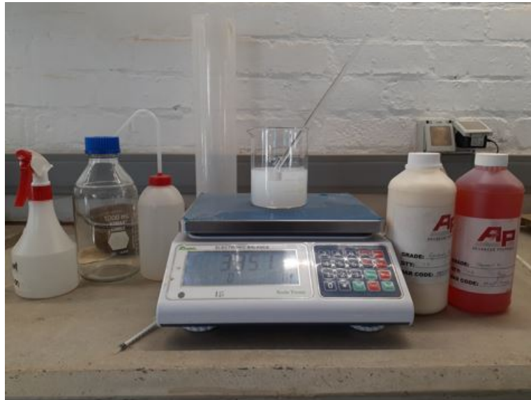
Figure 3.11: Terrasil+, Zycobond dust suppressant and their preparation
