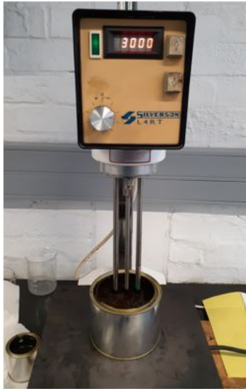
Figure 3.12: High shear mixing of bitumen and organosilane
