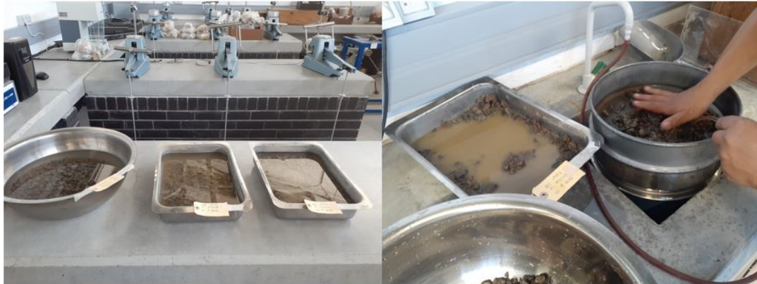
Figure 3.3: Washing of crushed stone in preparation of sieving
