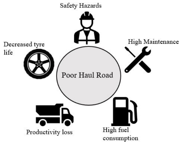
Figure 2.30: Cost impacts of poor haul roads.
