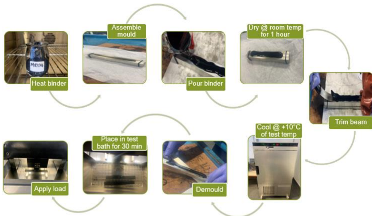
Figure 3.11: BBR Specimen Preparation
