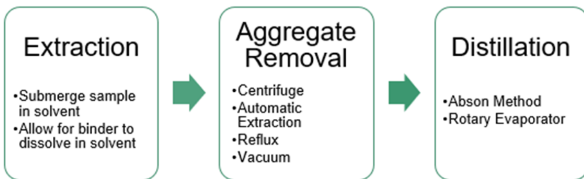
Figure 2.16: Binder Recovery Process
