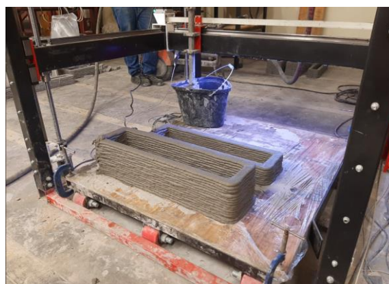
Figure 3-4: Procedure to incorporate the critical layer with various pass times
