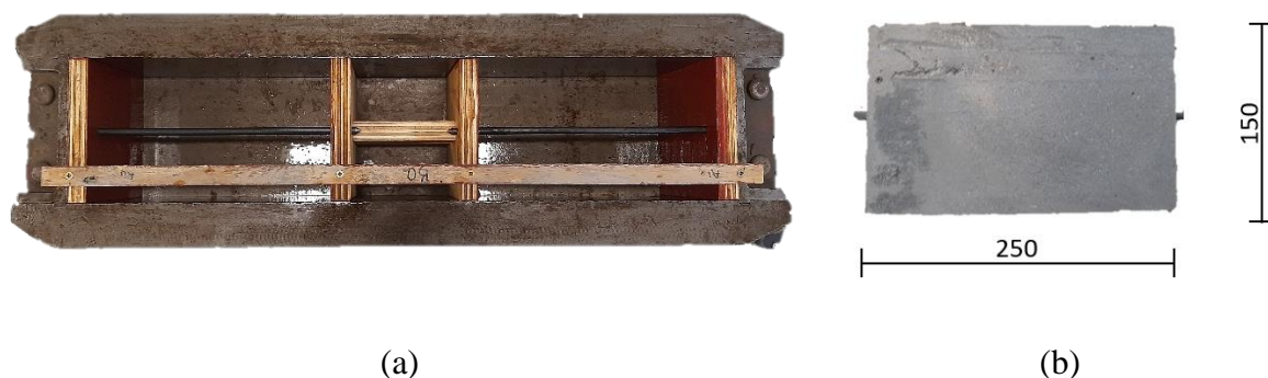
Figure 3-20: Steel mould and setup (a) for producing cast beams (b)
