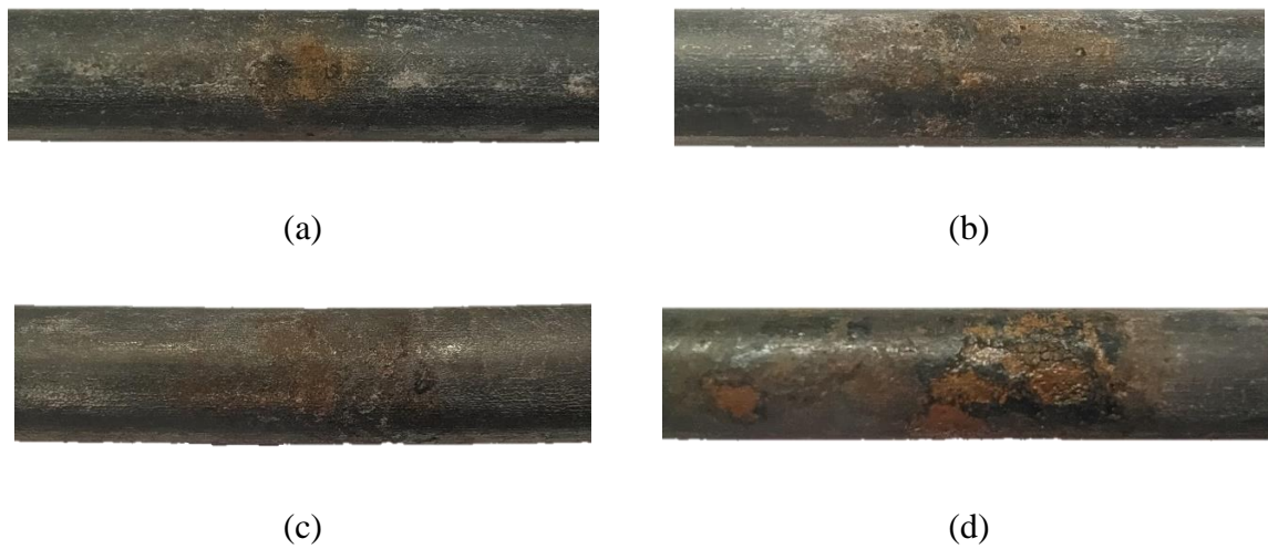
Figure 4-48: Pit formation at the critical layer for the 3D-0-2 (a), 3D-10-3 (b), 3D-20-1 (c), and 3D-30-2 (d) samples
