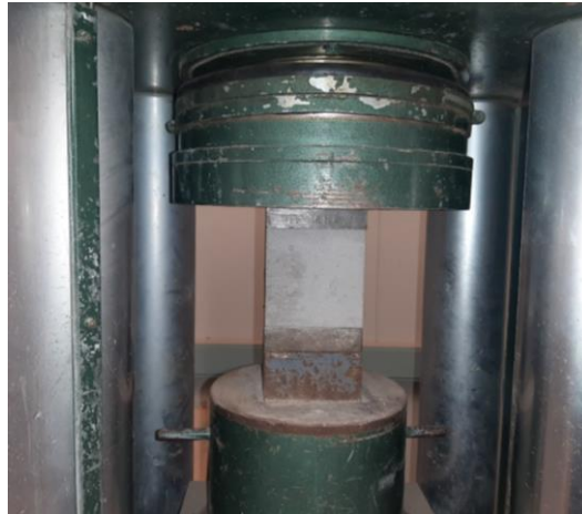
Figure 3-8: The Contest MTM compression test setup
