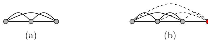
FIGURE 6.2: Graphical visualisation of the effect of meeting direct demand by adding a vertex to a route. The straight lines represent the road network and the curved lines represent the demand. In (a), a demand link is made to each other vertex in the route, while in (b), the effect of the inclusion of the red vertex is illustrated with respect to the direct demand met by all the other vertices, represented by the dashed lines.
