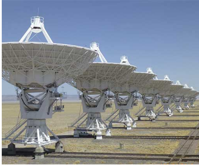
Figure 2.2: An array of radio telescopes known as the Very Large Array (VLA). Aside the MeerKAT in Figure 1.1, this is another type of radio telescope comprising of 27 dishes [17].
