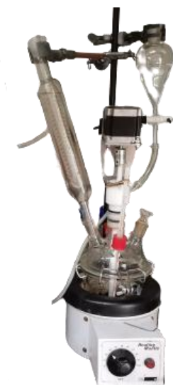
Figure 6. Experimental setup for one-pot phenolation and LPF synthesis.
