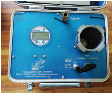
Figure 2.4. Pressure chamber used to measure SWP
