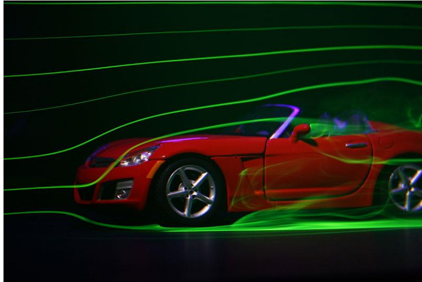
Figure 1.11: Visualization of the flow around the car with a thin layer along the body caused by the viscosity of the fluid. [104]
