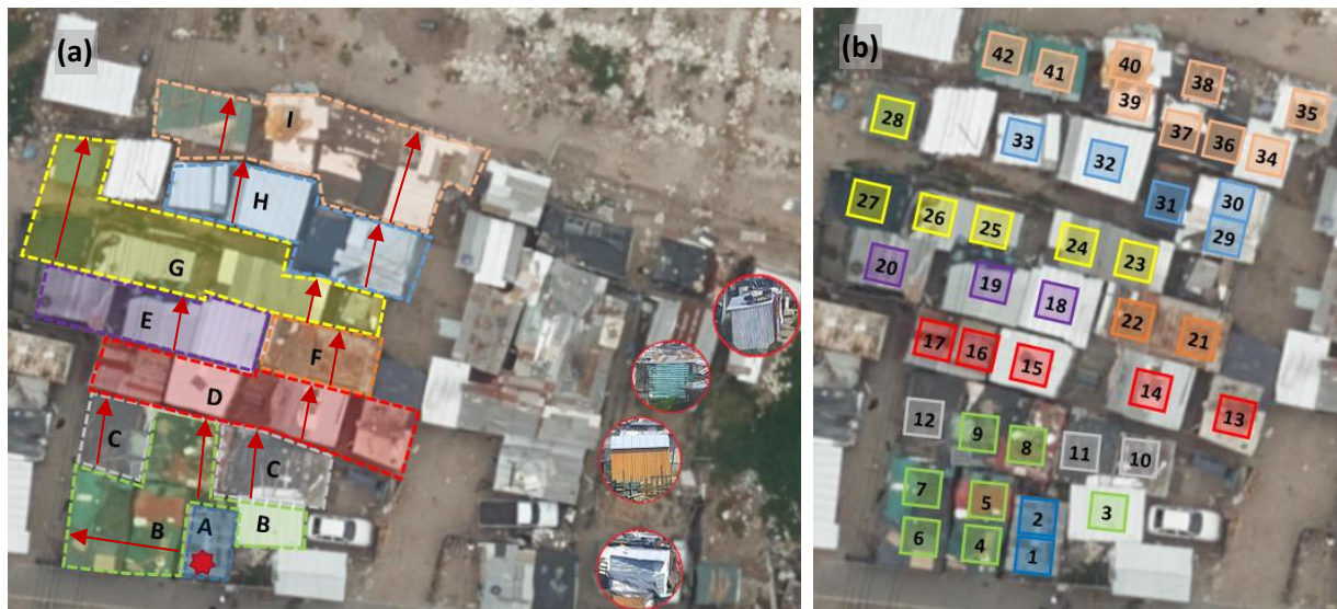
Fig. 5-4: Fire spread [116]. (a) Estimated fire line progress. The red star represents the dwelling of fire origin. The different zones, A to I, are associated with the fire line at different times. (b) Estimation of number of dwelling affected by the fire. Each number is associated to the colour of the corresponding zone (A to I).
