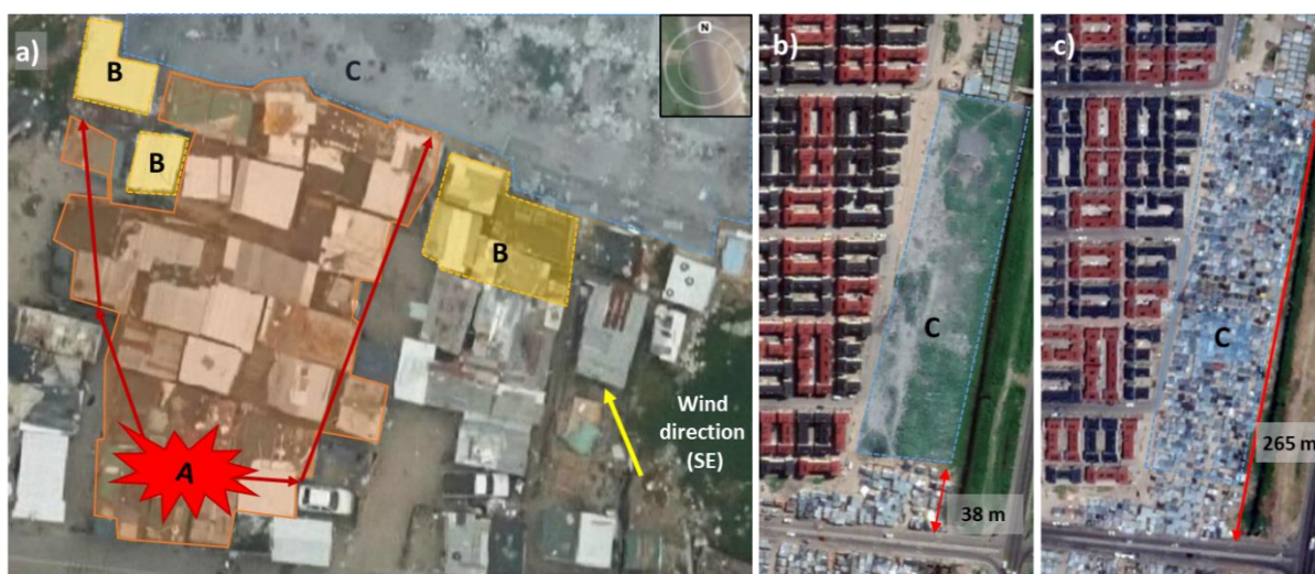
Fig. 6-5: (a) Fire pattern analysis CS1. The fire scar is shown in orange. The dwelling of fire origin is identified as being in Zone A. The fire pattern formation sequence is represented by the red arrows. Zone B depicts the dwellings at the north of the settlement that did not get burned. Zone C is the area with no combustible material. (b) A more detailed image of Zone C (image taken on 26/10/2020). (c) Zone C. The area has now multiple dwellings (image taken on 3/12/2020), the image highlights how rapidly such settlements can grow.
