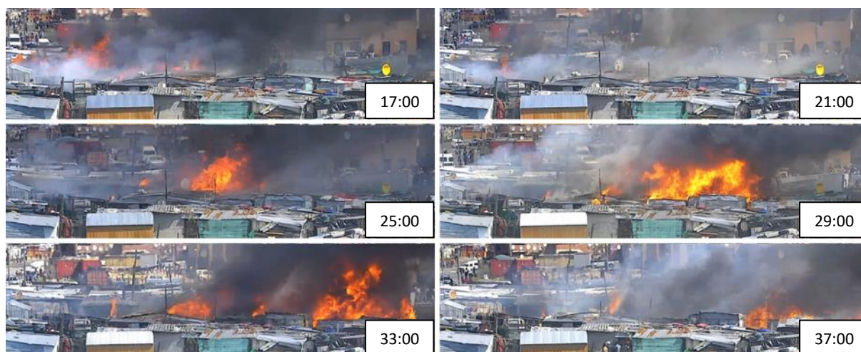
Fig. 5-9: Fire development from t=17:00 to t=37:00 . The fire intensity fluctuated due to the firefighters' interventions.
