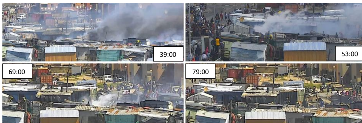
Fig. 5-10: Fire development from t=39:00 to t=79:00 . Fire extinguishment phase.
