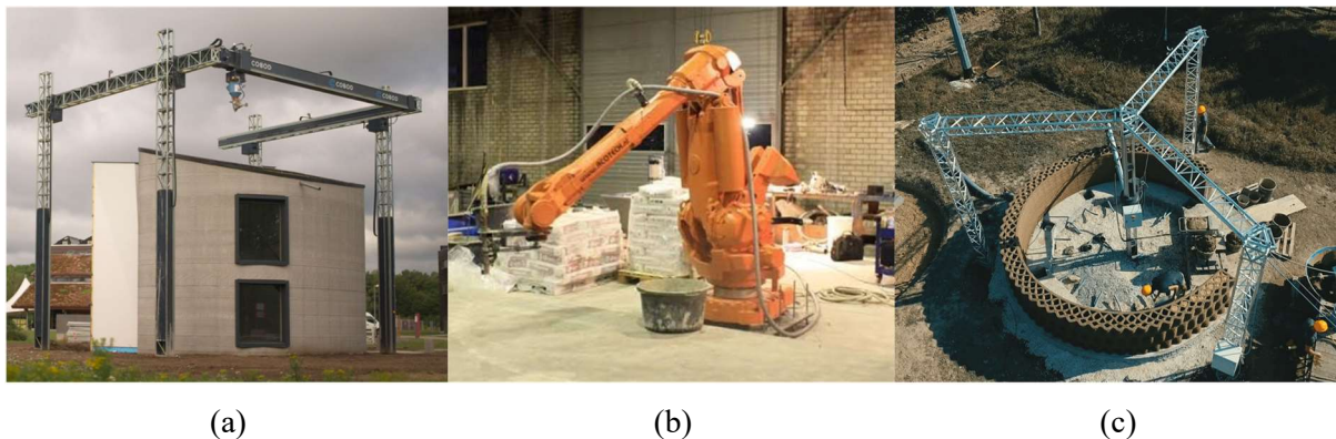
Fig. 2.3: 3D concrete printing systems, illustrating (a) gantry [19], (b) robotic [20], and (c) crane systems [21], respectively.
