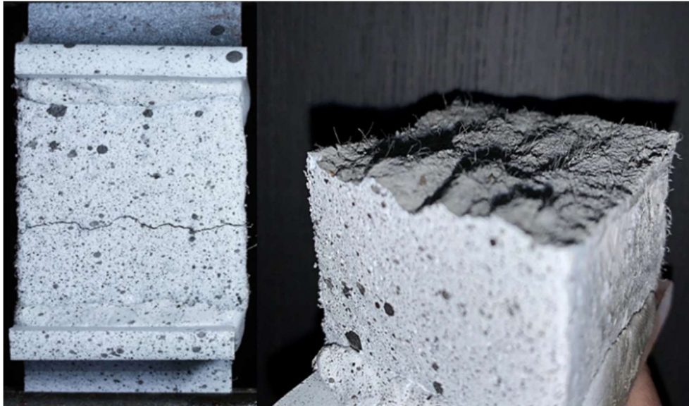
Fig. 3.18: illustrates the undulating tensile failure surface for specimens loaded in the transverse direction (D2).
