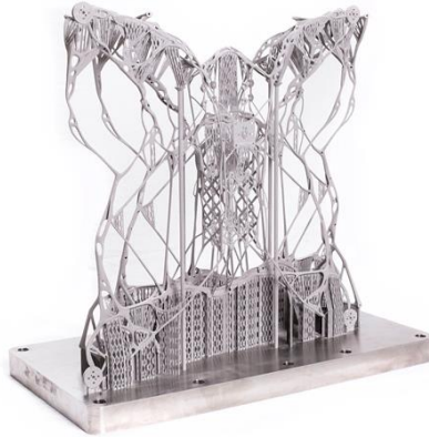
Figure A.2. Topology-optimised drone frame built using LPBF from Ti-6Al-4V (Aeroswift South Africa, 2018)
