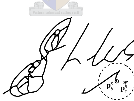
Figure 5.4: The locations of two disconnected endpoints \mathbf{p}_b^s (solid circle) and \mathbf{p}_c^h (x-marker) in a broken line. Candidate disconnected endpoints are within the vicinity of the dashed circle from \mathbf{p}_b^s .
