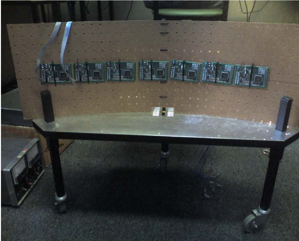
Fig 4.4 Devices under test suspended on the movable trolley
