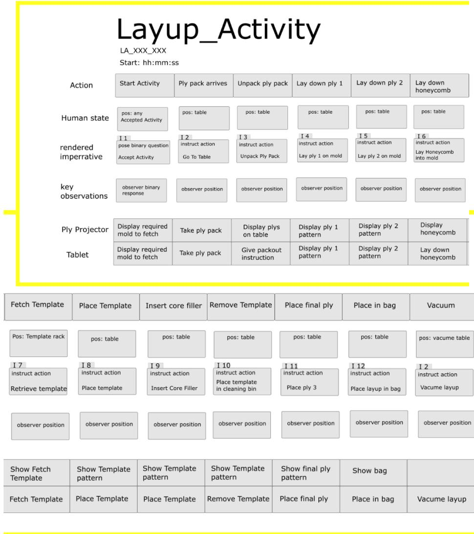
**Figure 78 – LUA action plan along with observations and imperatives to be rendered**
