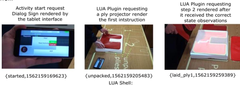
**Figure 46 – LUA in execution with the first three steps and their time stamps from the execution data block shown.**
