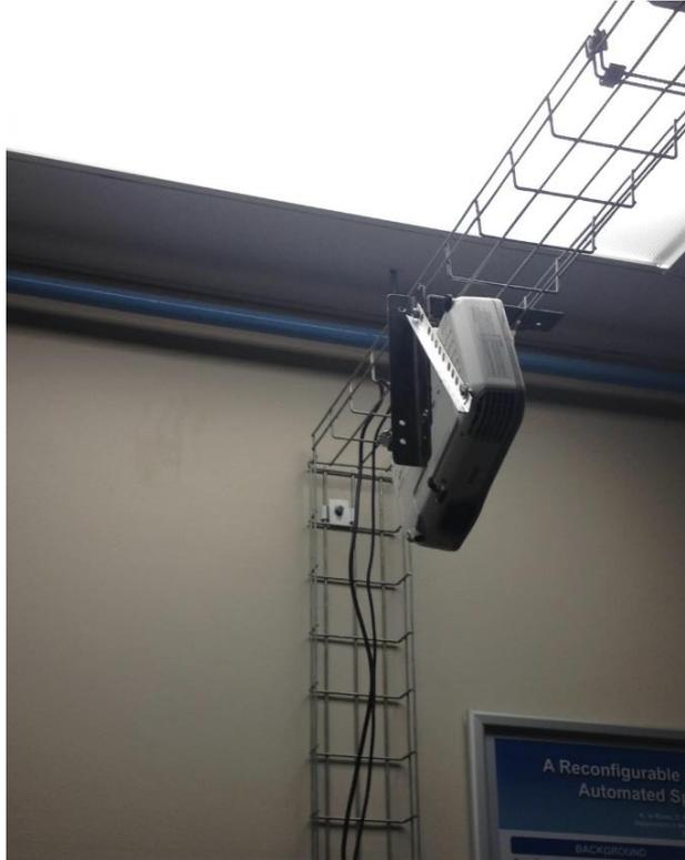
**Figure 77 – Projector mounted over the layup station connected to a Raspberry Pi 3 to act as the physical rendering component of the Ply Projector semiotic service holon**
