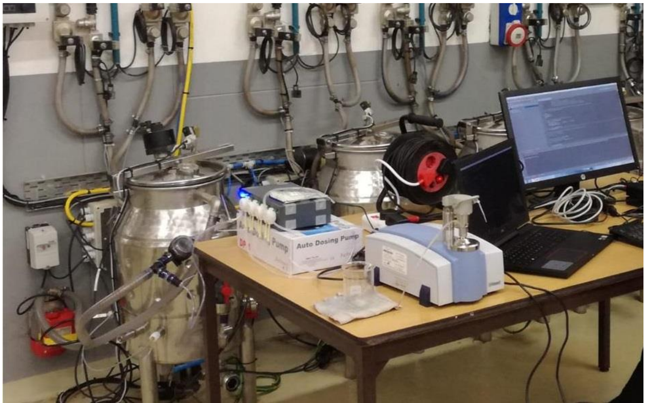
Figure 3.9: Position of Instrumentation and Sampling Pump
