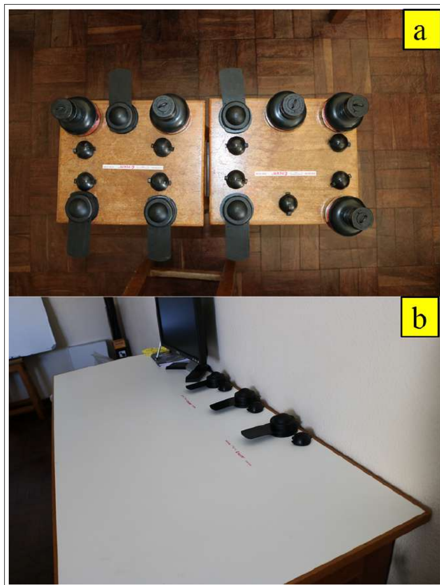
Figure 3.11: (a) Three LST-OO (EICs), two LLT-OO (EICs), two SST (EICs), and three SLT (EICs) were deployed in parallel with nine ParcRGMs. (b) Three sets of LST-OO (EICs) and ParcRGM were placed close to the wall ( <0.5 m).
