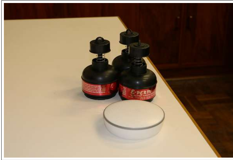
Figure 3.13: The Airthings™ radon detectors placed next to three short term electrets.
