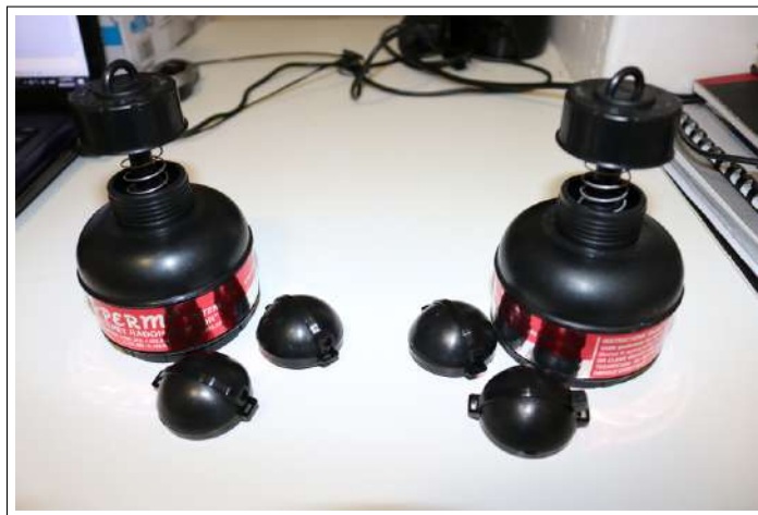
Figure 3.12: Two LST (EICs) and four ParcRGMs were deployed in parallel and placed next to one another.
