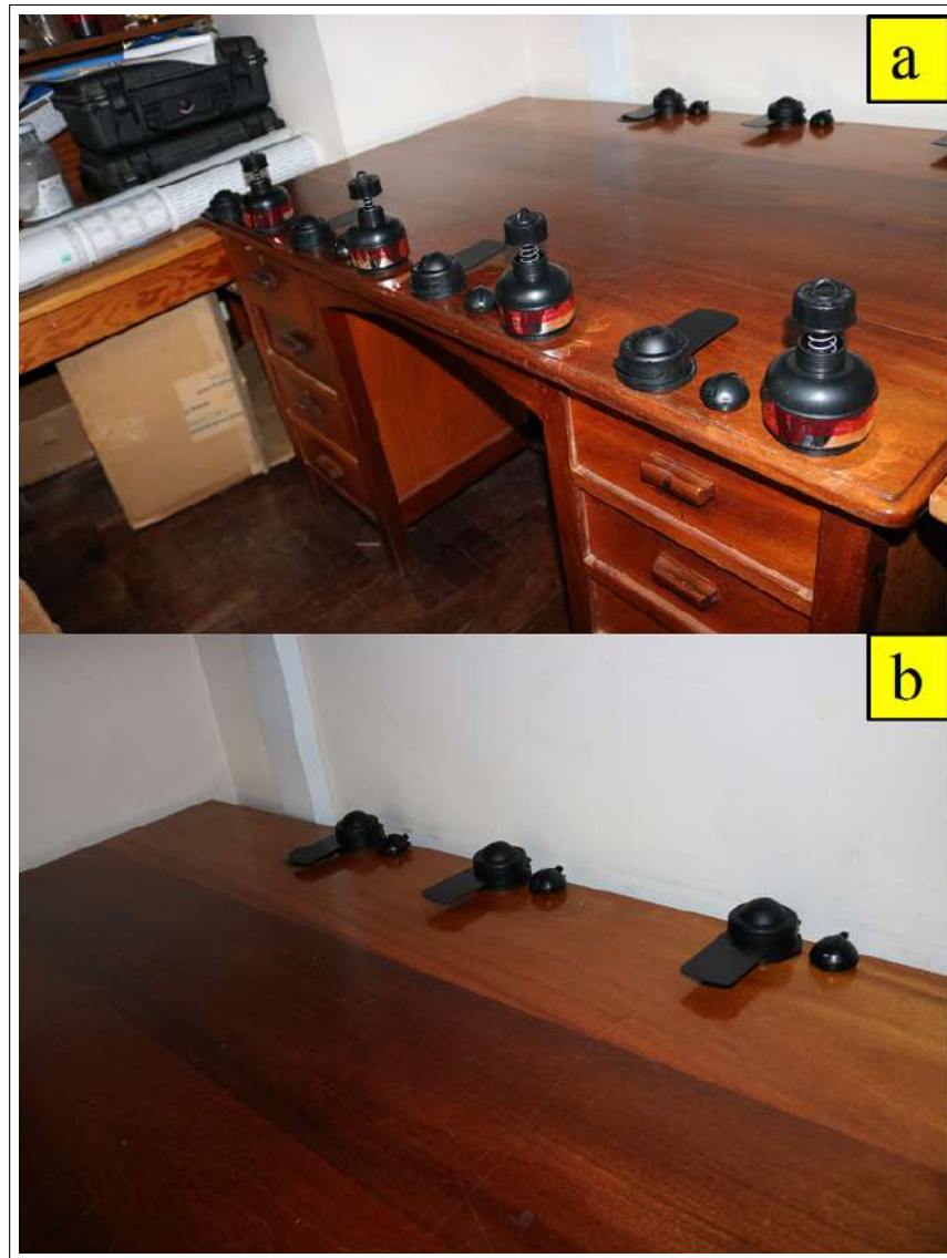
Figure 3.9: (a) Four sets of LST-OO, SLT (EICs) and ParcRGMs were deployed in parallel and placed away from the wall ( >0.5 m). (b) Three sets of LST-OO and ParcRGM were deployed in parallel and placed next to the wall ( <0.5 m).
