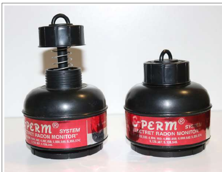
Figure 3.2: Left, E-PERM (S-chamber) in opened position. Right, E-PERM in closed position.
