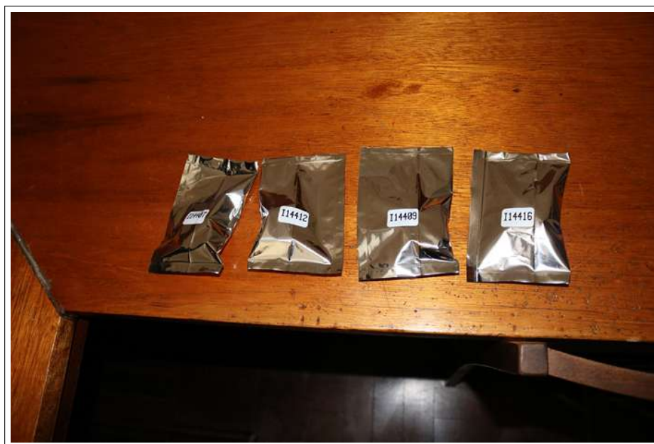
Figure 3.4: The ParcRGMs inside the radon-proof bags.
