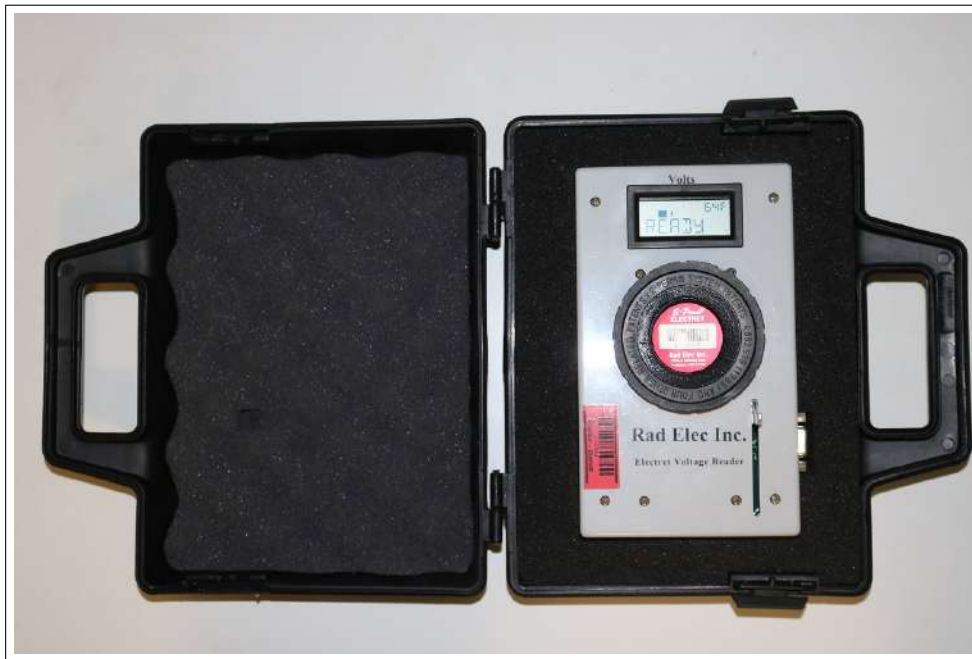
Figure 3.1: Voltage reader used for measuring initial V_i and final V_f voltages from the electrets.
