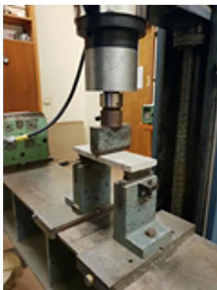
Fig. 3-3 Geopolymer boards being tested for flexural strength (3-point bending)
