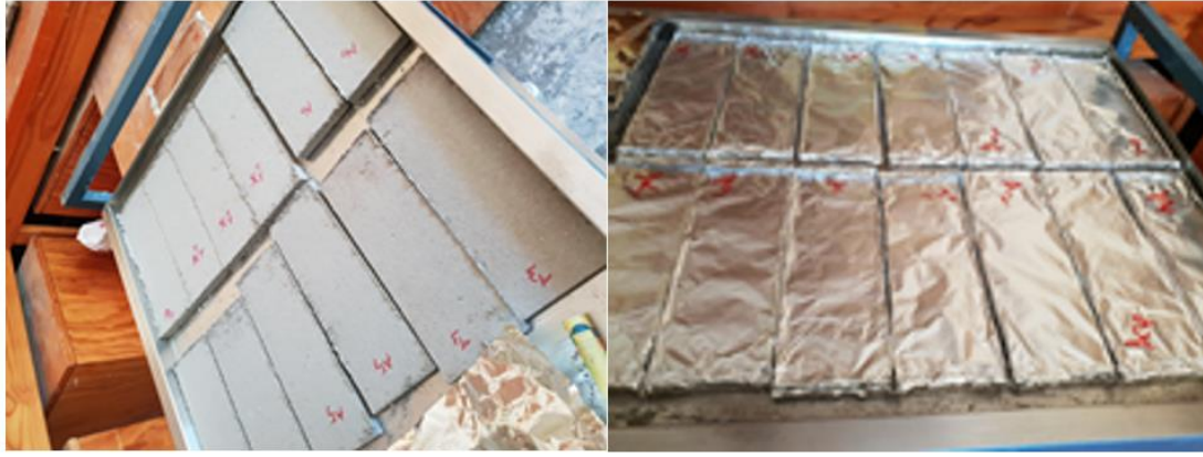
Fig. 3-2 Geopolymer boards wrapped with aluminium foil prior to curing
