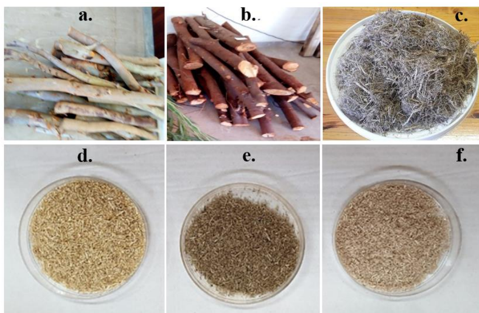
Fig. 3-1 Lignocellulose materials as received and after milling (a) A. mearnsii (b) A. saligna (c) bagasse (d) A. longifolia particles (e) bagasse particles (f) A. mearnsii particles.
