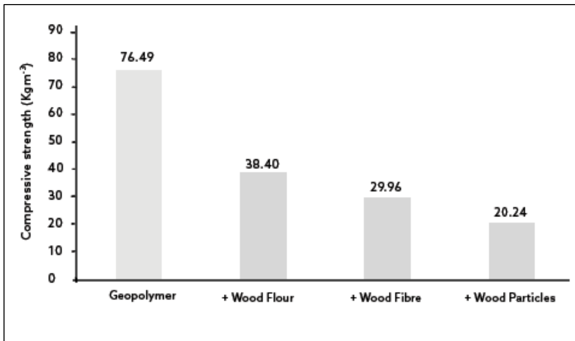
Fig. 2-5 Effects of wood aggregates on the compressive strength of geopolymer composites (Source: Sarmin (2016))
