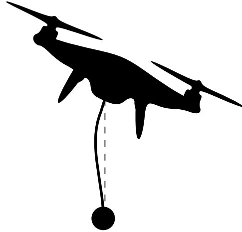
Figure 2.2: Multirotor carrying a suspended payload 1 .
