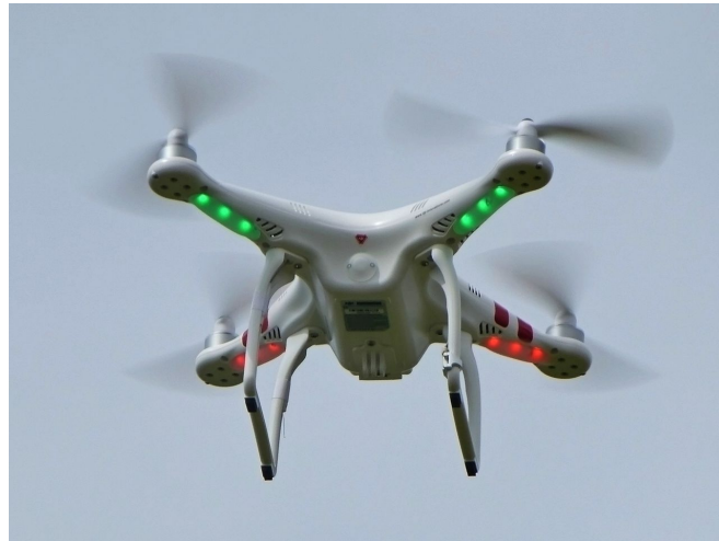
Figure 1.1: A quadcopter, which is a subset of multirotors, hovering in the air.
