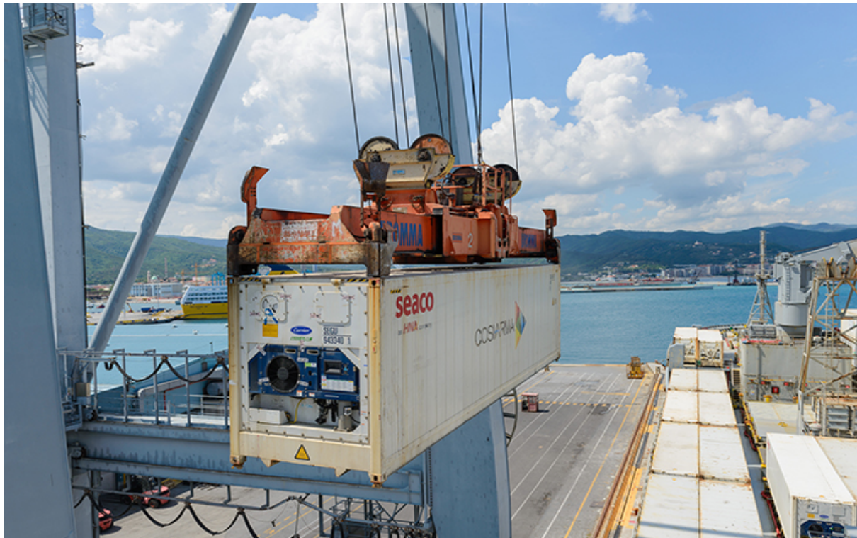
FIGURE 2.5: Example of a reefer container used for citrus shipments [100].
