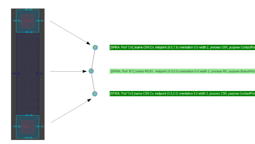
Figure 4.6: Simply geometry to undirected graph example
