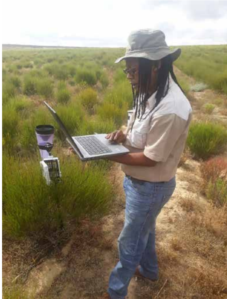
Figure 3.8: Em 50 ECH2O data logger used for collection of the soil water content data from the ECH2O 5TM and ECH2O EC-20 sensors. The figure shows the downloading of soil water content data in progress from the field.
