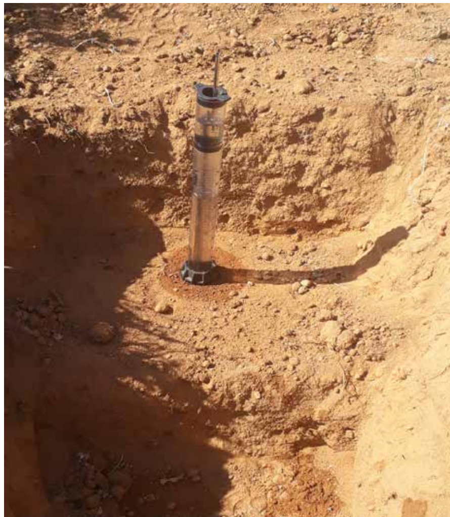
Figure 3.6: A Minidisk Infiltrometer from Decagon Devices was used to measure unsaturated hydraulic conductivity in situ .
