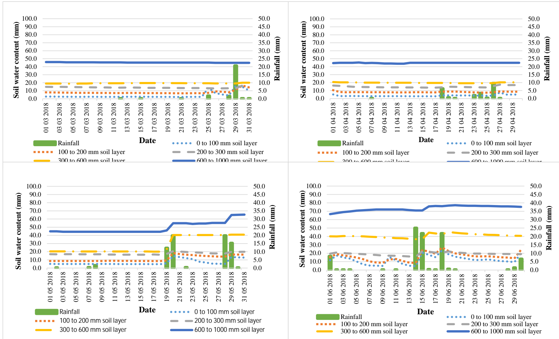
Figure A3-6: Soil water content and rainfall of Meulsteenvlei (from March 2018 to June 2018).
