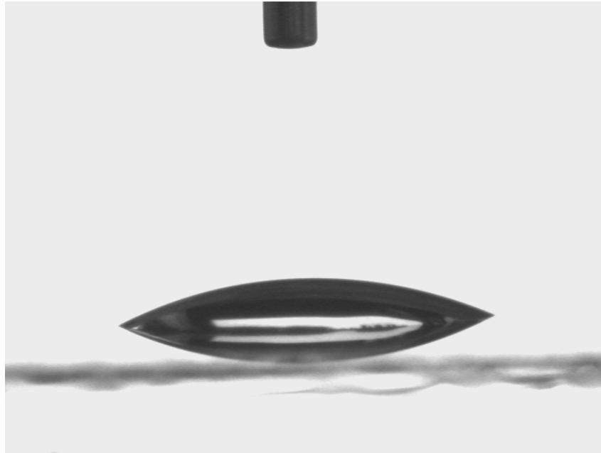
Figure 4.2: Imaging of the 1\mu\text{l} droplet on a hydrophilic area on sample M19
