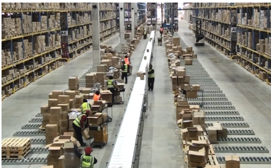
(a) The unidirectional cyclical picking line in the Cape Town DC.
