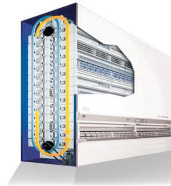
(b) A unidirectional vertical carousel illustration. Source: Nicolas et al. [87].
