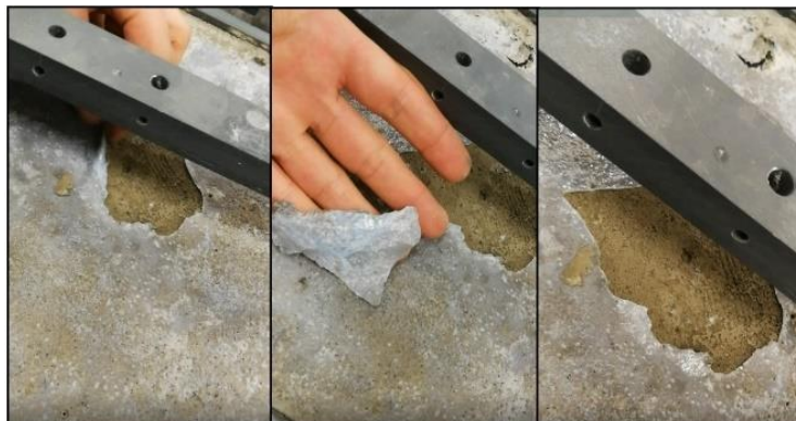
Figure 4.15: Layer created by the petroleum curing agent (CA2)
