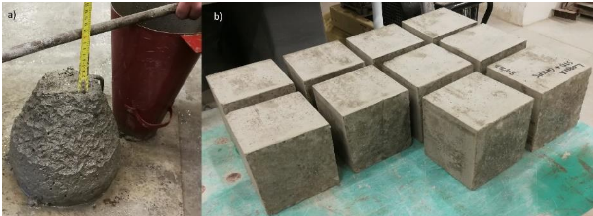
Figure 3.1: a) Slump test b) Cube strength samples
