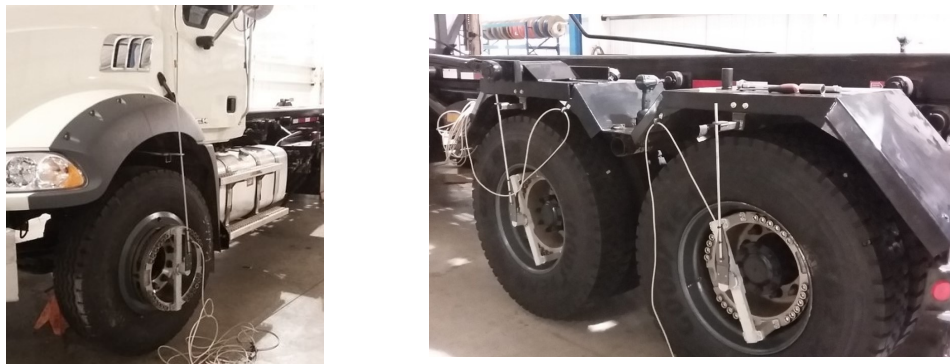
(a) Front wheel force transducer setup. (b) Rear wheel force transducer setup.
