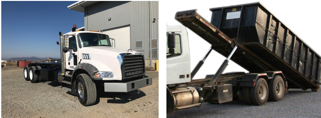
(a) Similar truck model (My Little Sales- man, Inc., 2019). (b) Roll-off mechanism (Wikimedia Com- mons, 2019).
