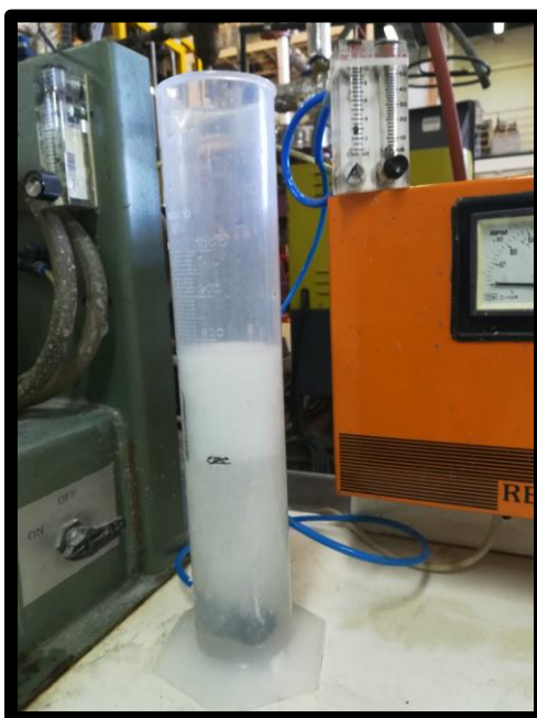
Figure 15: Froth stability and froth height experiment in measuring cylinder
