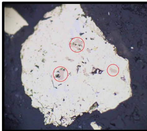
Figure 23: Image of a pyrite grain with pyrrhotite inclusions, highlighted with red circles
