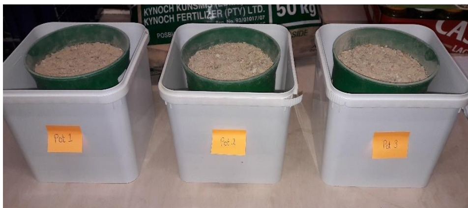
Figure 3.1: Pots were placed in 5 L ice cream buckets filled with 1 L of water. Capillary action was used to determine the field capacity of the sand medium.
