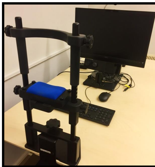
Figure 7. The physical setup of the EyeLink® 1000 Plus eye-tracker in Stellenbosch University’s MutliCog Laboratory
