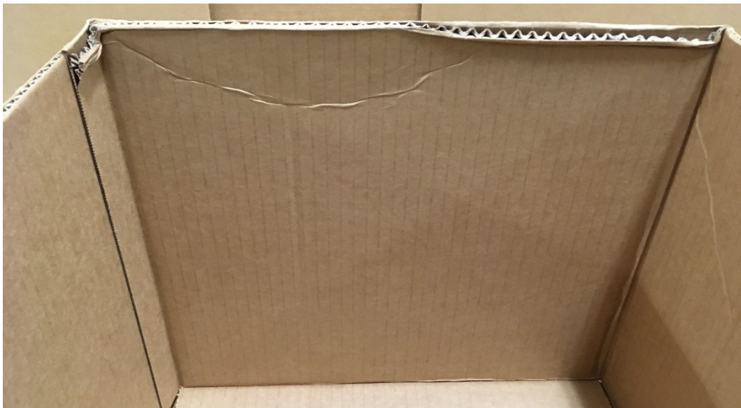
Figure 4.8: Delamination damage of the Mk 4 telescopic carton observed in boundary condition test case (3)
