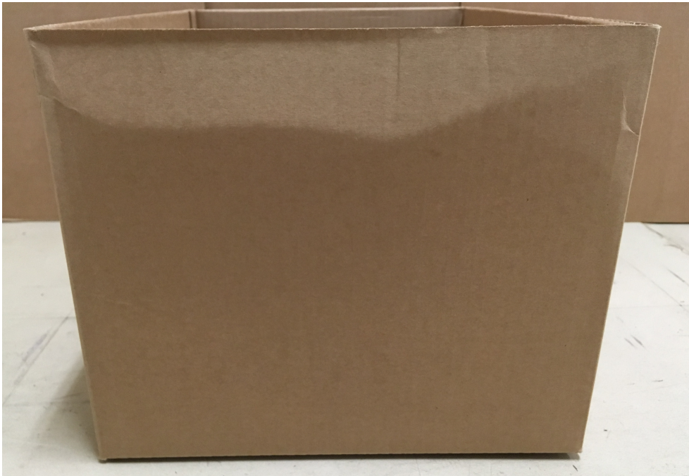
Figure 5.12: Crease lines in the corners of the Mk 4 inner after compression
