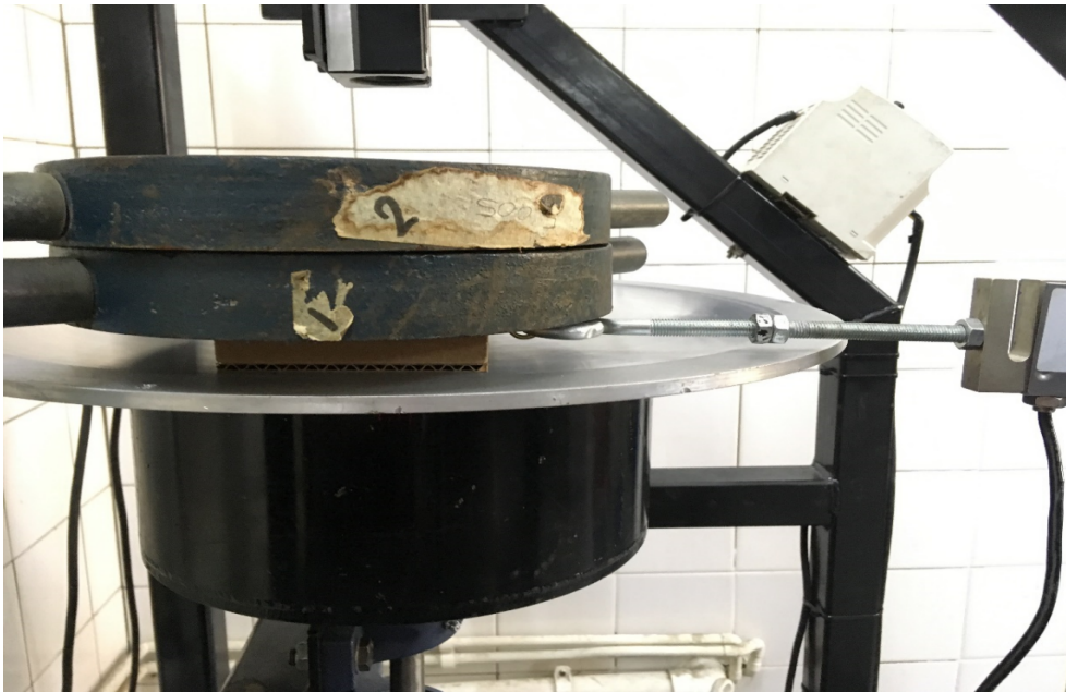
Figure 4.1: Friction coefficient experimental setup
