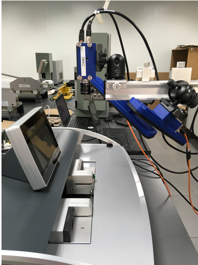
Figure B.4: Tensile test and DIC setup
