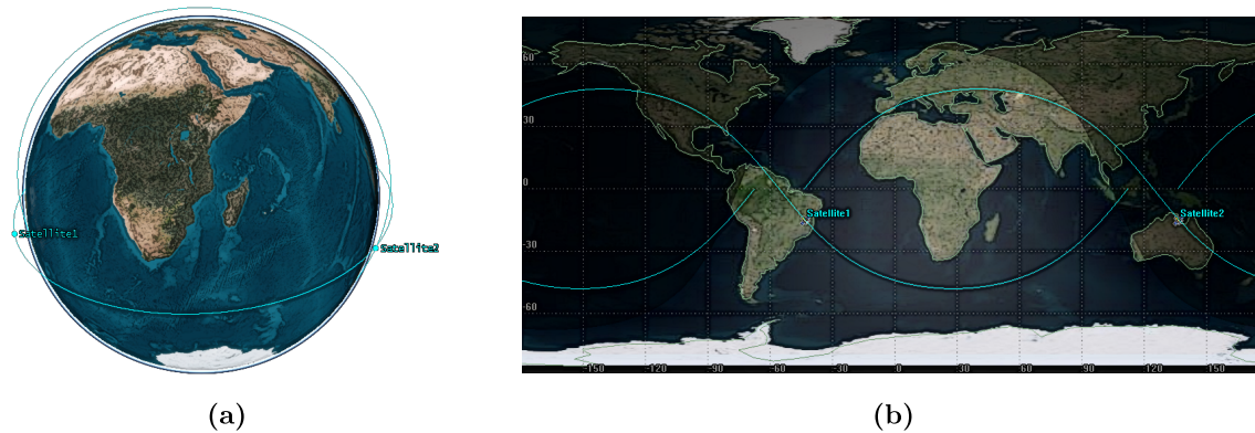
Figure 4.15: Orthogonal RGT orbit planes to reduce DG. (a) shows the satellites orbiting Earth and (b) is its projection onto a 2-D plane.
