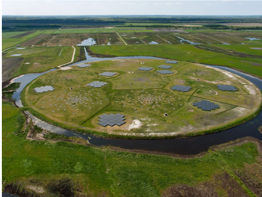
FIGURE 1.1: The LOFAR antenna array, a pathfinder for the SKA, operates at the lowest frequencies observable from earth. LOFAR consists of 50 Stations across Europe, with the core (38 stations) concentrated in the Netherlands [17].
