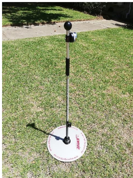
Figure 2.3: Visual image of the rising plate meter.
