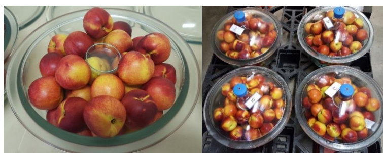
Figure 4.1.1. Illustration of 'August Red' nectarines placed in 14 L desiccators for ethyl formate fumigation and phytotoxic assessment trials during the 2015/2016 season.
