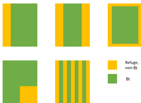
Figure 2.7: Different possible structured refuge layouts. From top left: linear block, bracket, border, block, and strips. Recreated from an illustration by Aroian [3].
