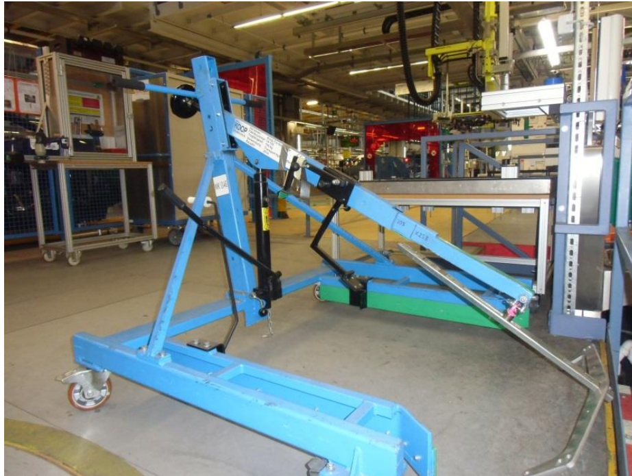
Figure 91: Manual hoist to remove a damaged battery from a unit
