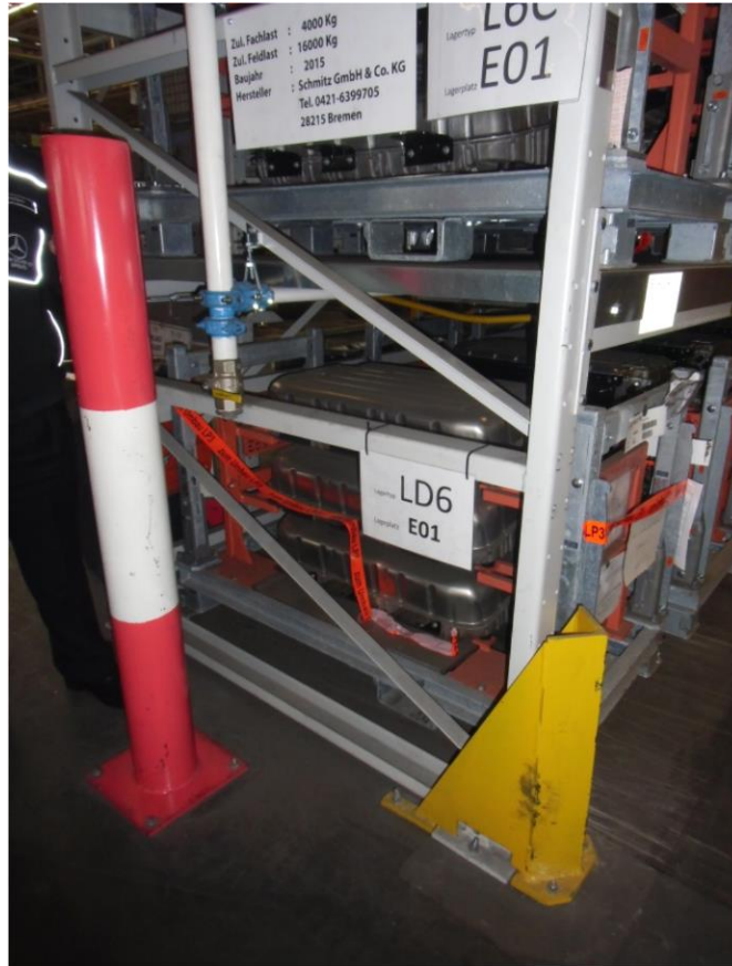
Figure 95: Guarding poles in the warehouse to prevent HV battery damage
