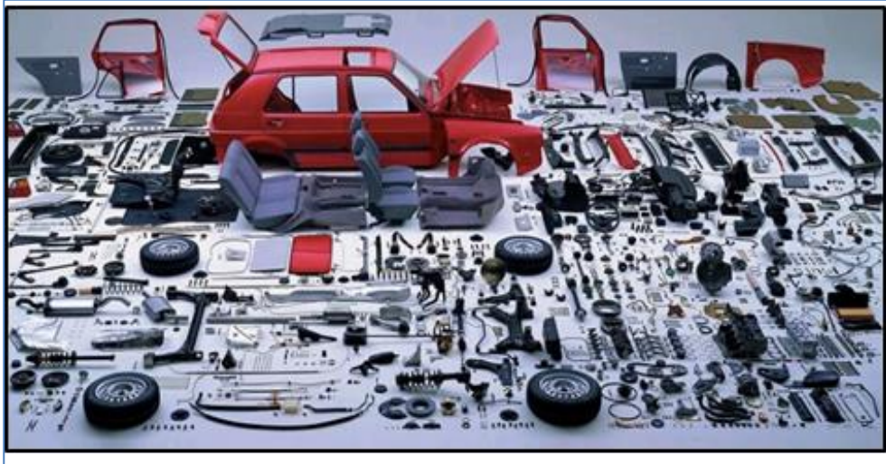
Figure 32: Exploded view of the 1983 Volkswagen Golf MK2 (Adapted from [212])
