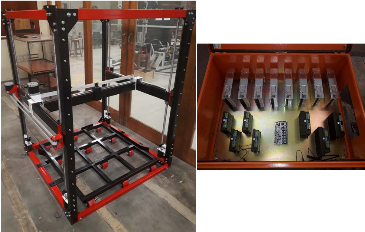
Figure 2.6: The completed 3D concrete printer with automation system (left) and the electrical control box (right).
