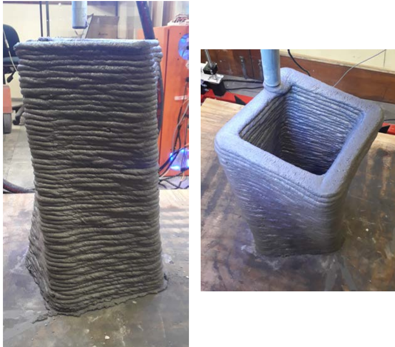
Figure 2.12: A 250 x 250 x 700 mm square hollow column that twists 45° over its height.
