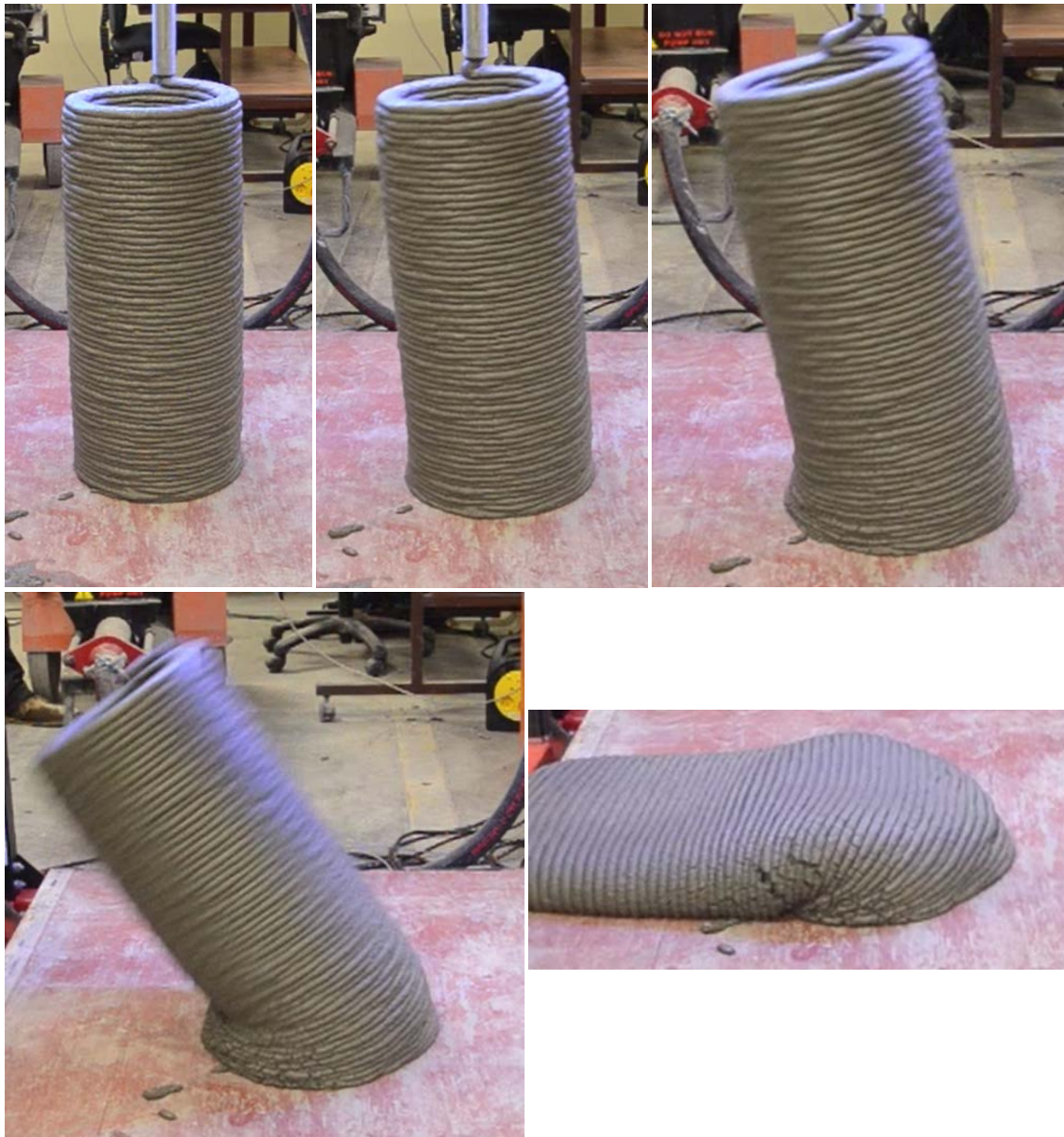
Figure 5.21: Failure progression of the column clearly indicates plastic yielding of the bottom layers.
