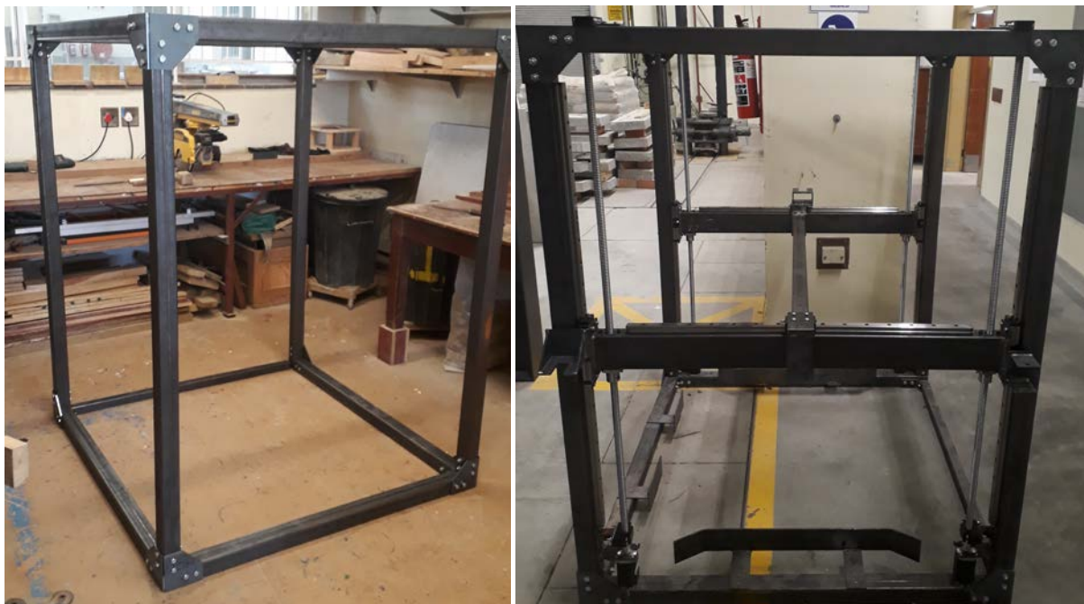
Figure 2.5: Manufacturing of the 3D concrete printer indicating the framework (left) and the almost completed mechanical component of the printer (right).
