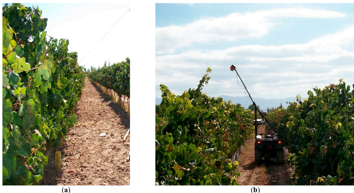
Figure 1. (a) Example of a vertically shoot positioned (VSP) vineyard (cv. Malbec); (b) Tetracam ADC multispectral camera mounted on a boom on a quadricycle in preparation for a nadir-viewing capture on the canopy in a VSP vineyard.
