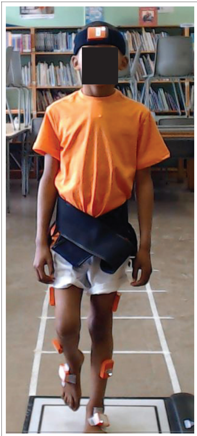
FIGURE 1: Placement of the Xsens sensors on a participant.
