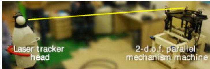
Figure 2.2: Laser tracker used for calibration (Jeon et al. , 2010).
