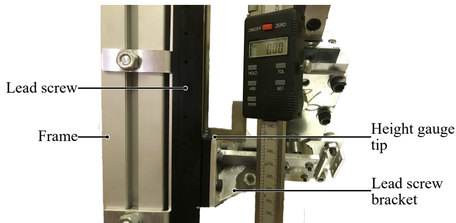
Figure 6.2: Height gauge measuring the change in pivot point height on the lead screw bracket.
