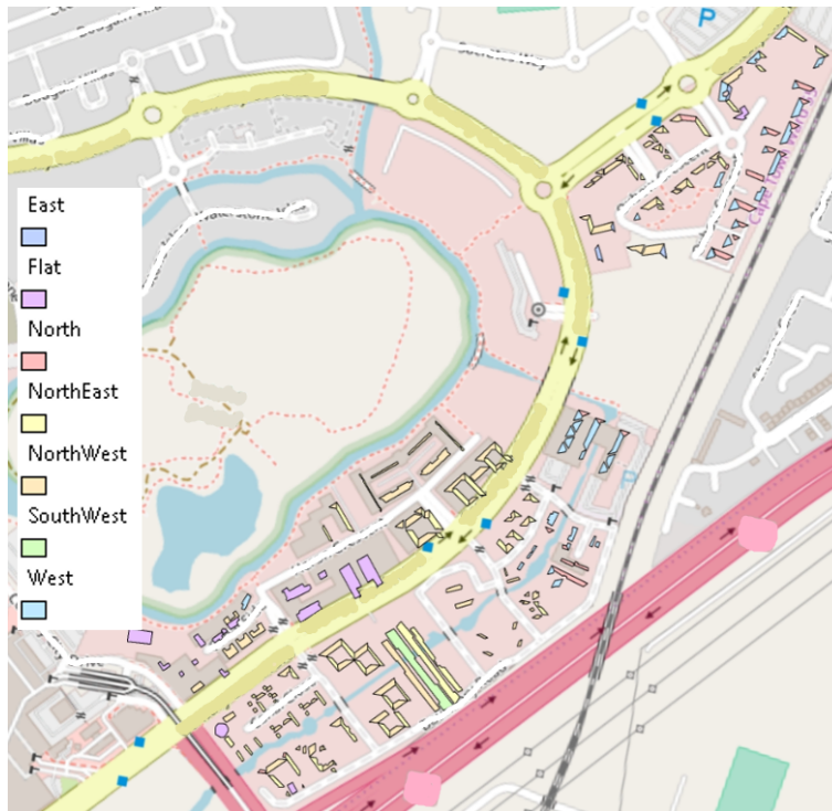
Figure 4.11: Example of Polygons Indicating Roof Space with PV Potential in Commercial Area
