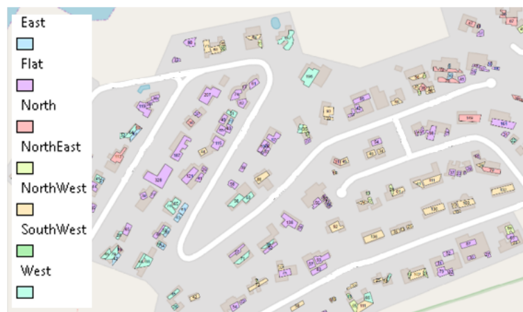
Figure 4.10: Example of Polygons Indicating Roof Space with PV Potential in Residential Area
