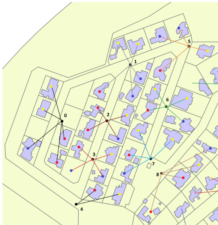
Figure 4.6: Example of Residential Network LV Kiosks
