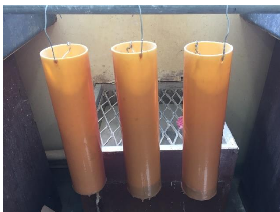
Figure 3.15: Liquid latex on PVC pipes
