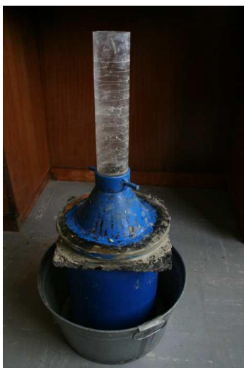
Figure 2.31: Laboratory Marvil permeability test setup (Annandale, 2012)
