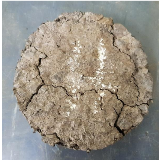
Figure 4.2: Cracked surface of Core H noted during visual inspection
