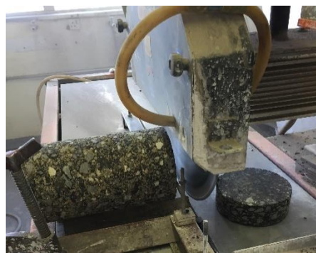
Figure 3.10: Sawing of asphalt core
