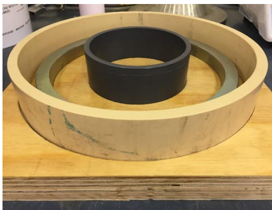
Figure 3.13: Manufactured mould frame
