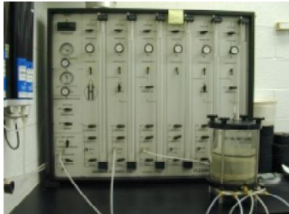
Figure 2.27: Constant head permeameter (Maupin, 2000)
