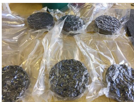
Figure 3.11: Vacuum-sealed asphalt cores
